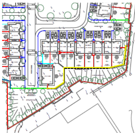
Extract from Drawing No. 5 – Proposed Site Plan – Boundary Treatments (4m high retaining wall coloured yellow)
